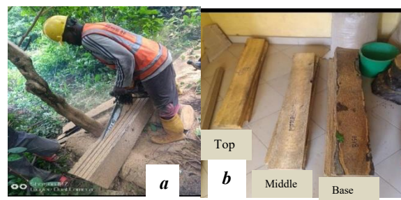
Plate 1: Conversion and Sorting (a) sawing process (b) Sorted lumber from the base, middle and top sections
